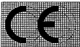
If the CE marking is reduced or enlarged the proportions given in the above drawing must be respected.
